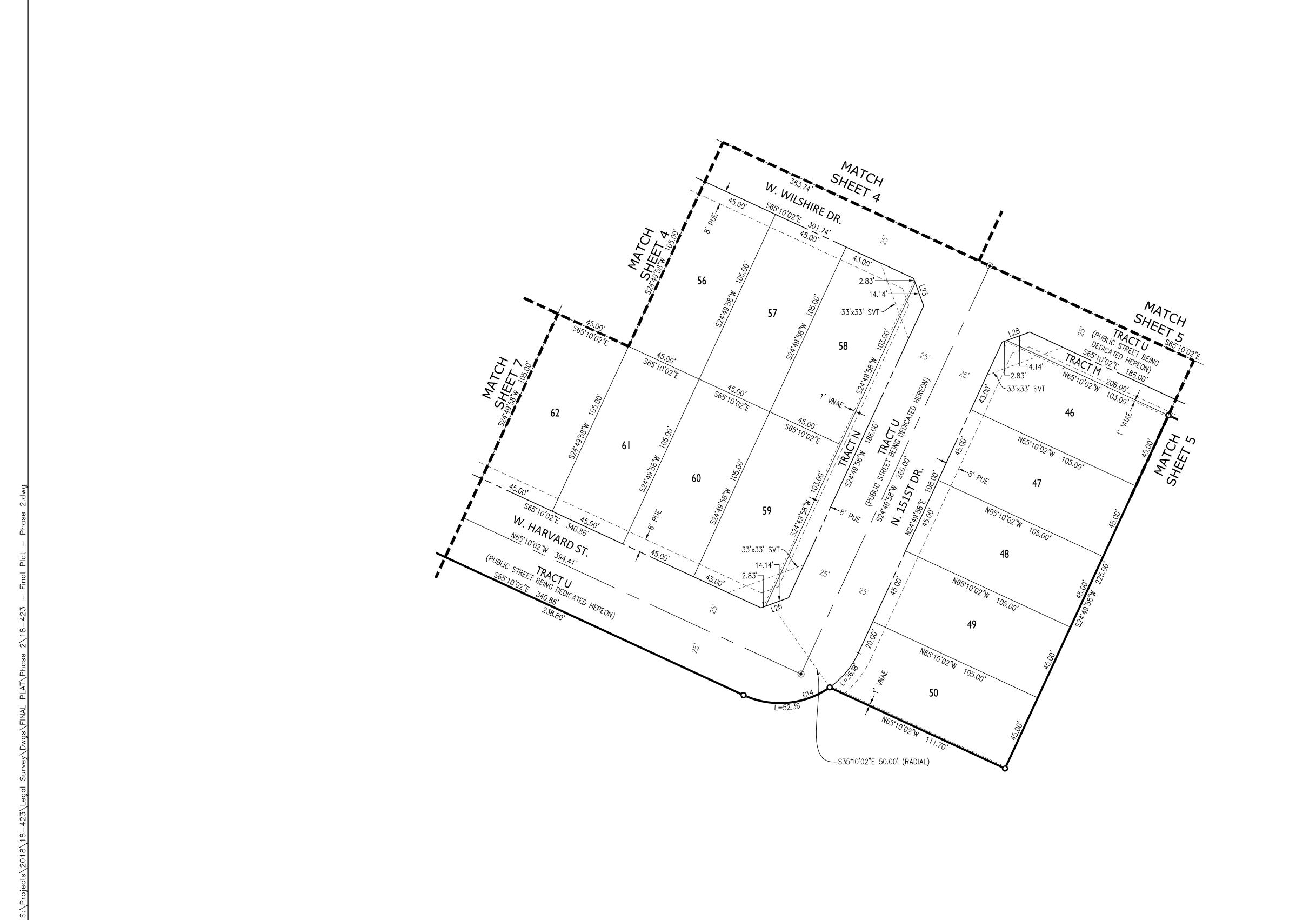
LEGEND FOUND MONUMENT AS NOTED SET BRASS CAP AT COMPLETION OF CONSTRUCTION CORNER OF SUBDIVISION, SET 1/2" REBAR W/CAP #21071, OR AS NOTED OTHERWISE. REGISTERED LAND SURVEYOR PUE PUBLIC UTILITY EASEMENT RIGHT-OF-WAY WSE WATER SERVICE EASEMENT USE & BENEFIT EASEMENT SWE SIDEWALK EASEMENT PRIVATE SIDEWALK EASEMENT PSWE PRIVATE DRAINAGE EASEMENT PDE WATER LINE EASEMENT VEHICULAR NON-ACCESS EASEMENT SIGHT VISIBILITY TRIANGLE PRIVATE STREET PLAT BOUNDARY
