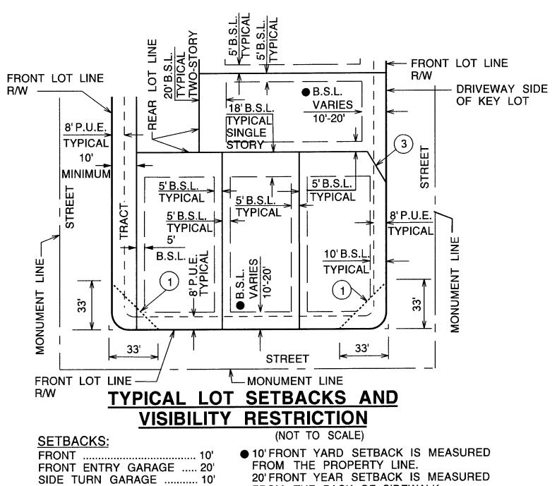
● 10'FRONT YARD SETBACK IS MEASURED FROM THE PROPERTY LINE. 20'FRONT YEAR SETBACK IS MEASURED FROM THE BACK OF SIDEWALK. 20'FRONT FACING STANDARD GARAGE 10'SIDE-TURN GARAGE 10'PORCH/LIVING AREA
